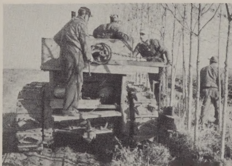
TREE PLOW & ROOT PRUNER - A "U" shaped blade alongside the Caterpillar tractor cuts off the roots and also lifts up the trees and plants.
